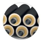
Pipes with combined insulation for construction of trunk oil and gas pipelines as well as process pipelines which carry high temperature medium up to 680 °F. Made from basalt fiber and polyurethane foam.
