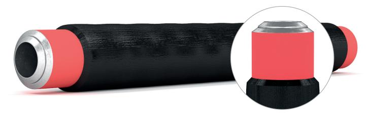
Metal-plastic pipes and connection pipes with a diameter Metal-plastic pipes and pup-joints with diameter up to 12.8 in. with maximum wall thickness of 0.87 in. represent a steel pipe, a pup-joint pipe with polyethylene (for underground routing) or paint coating (above-ground routing), lined with polyethylene pipe (shell) on the inside and fixed with tips made of:
